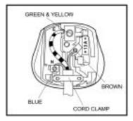
• Connect the green and yellow (earth) wire to the terminal in the plug which is marked with the letter "E" or the earth symbol (+) or coloured green and yellow.
